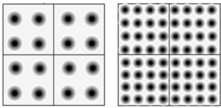
To send data faster – we need to have more bits sent per cycle – thus we need smaller targets. As we move to faster and faster data rates – the targets get smaller – and we can't send as far and still be accurate. We can go from 2 targets (BPSK) to 4 targets (QPSK) to 16 targets (16-QAM) to 64 targets (64-QAM)
